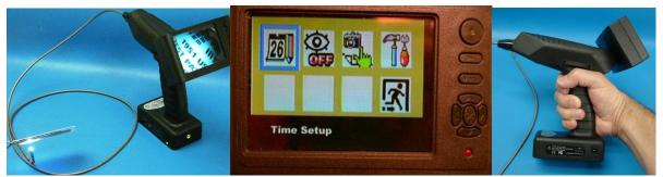
3.9mm Pistol grip two-way articulating videoscope, great resolution, built-in led lamps in tip rated at over 10,000 hours of light, with variable light settings. Unit is lightweight, rugged, easy to use and rechargeable! 1 year warranty
